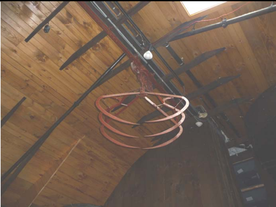
Detail of hayloft pulley system.
